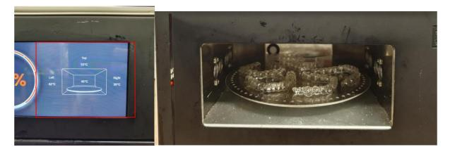
Temperature has a tangible effect on the material and output of an LED light. In general, the cooler the environment, the higher an LED's light output will be. Higher temperatures generally reduce light output and therefore, affects the curing process.
