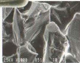
The patented Radiance mechanical lock base shown here at 24X magnification (left) and at 1000X magnification (below) allows for a strong bond in the center of the pad and a weaker bond on the edges for easy and predictable debonding.
